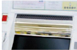
Mirror Allows the ATM user to view the situation behind them
