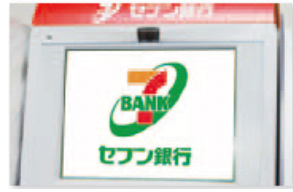
Secondary display Screen display used for advertisements and warnings
